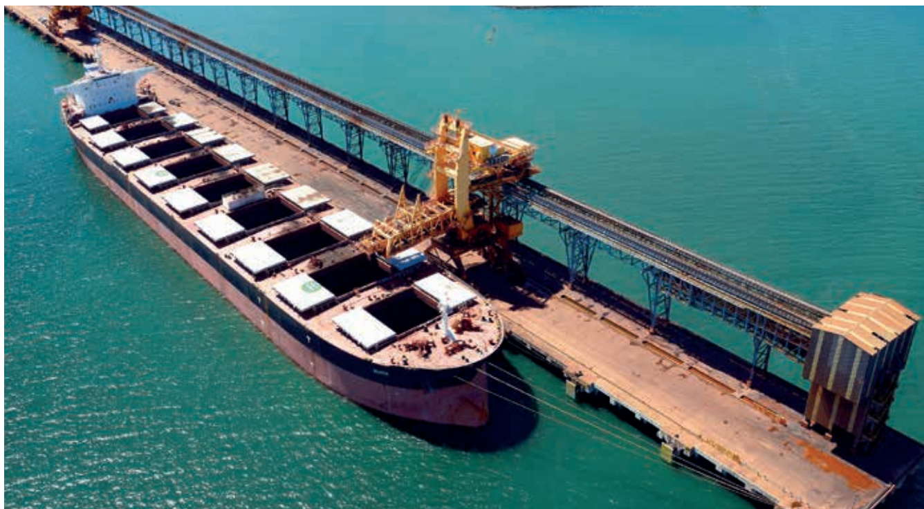
Iron ore loading at Impala Terminals and Mubadala's Porto Sudeste export facility in Brazil.
