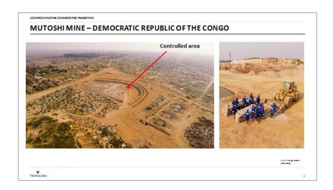
The picture on the left here shows how a designated area has been fenced in, and the over-burden within the perimeter removed. Miners are organised into a licensed co-operative, trained and provided with protective equipment.
